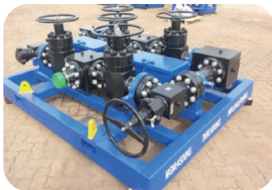
Well testing manifold in Saudi
